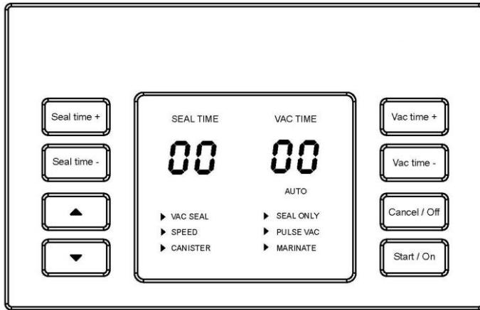
**Seal time +** : Button to increase the sealing time
