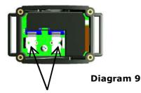
Reset: connect the 2 supports of the battery
